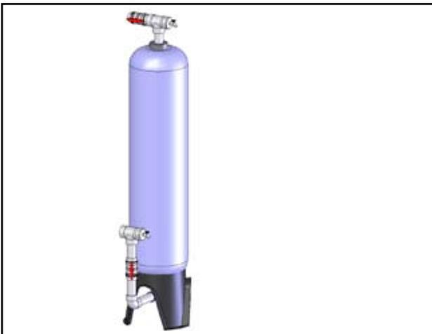
Connect the inlet and outlet plumbing according to your preferences and any applicable local codes. Include sample/drain ports with hose-bibb connections on the inlet and outlet piping to facilitate startup and service.
