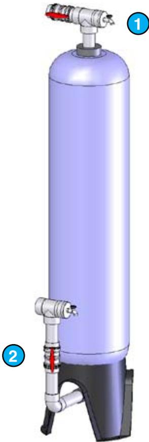
1. Connect a hose to the hose bibb on the outlet of the tank. Run the hose to a drain.
