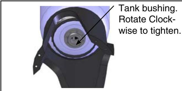
Lay the tank down and check the bushings on the inlet and outlet (bottom and top) of the tank. It is common for them to loosen during shipment. Tighten the bushings with a strap wrench as needed
