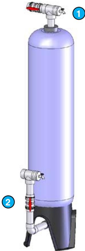
1. Connect a hose to the hose bibb on the outlet of the tank. Run the hose to a drain.
