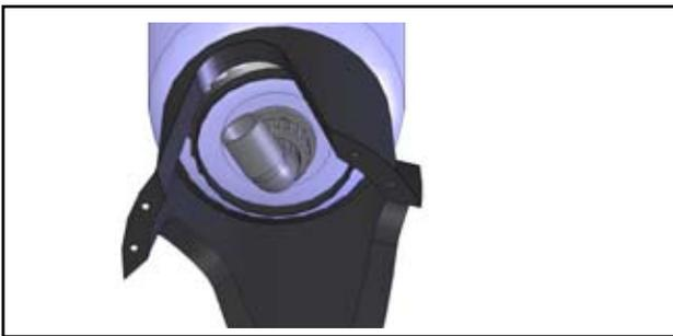
Connect the Union fitting to the inlet bushing (bottom)
